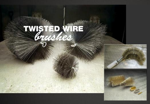
Twisted wire brushes are made by taking two steel wires (in galvanised or stainless steel), placing brush fibres between them and twisting them tightly. These brushes can be manufactured from a wide variety of fibres and are designed to clean hard-to-access conduits and cavities. Application areas include food, the automotive industry, cosmetics, bottling, pharmacology, plumbing and laboratory research.
