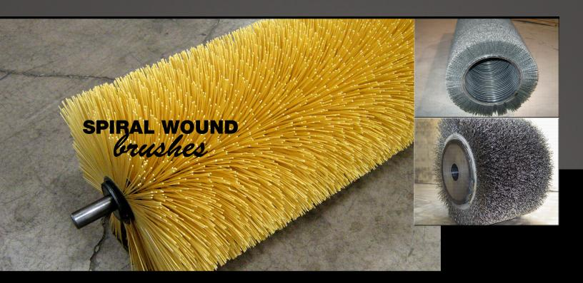
This type of brush roller is constructed from a strip brush that is wrapped around a metal core or directly onto a shaft. It's best suited to very small or very large diameters. The spacing between each coil makes it possible to adjust the brush's density according to your application. With little space between the coils, a very dense cylinder brush is obtained; with wider spaces, there's a slacker coil.
